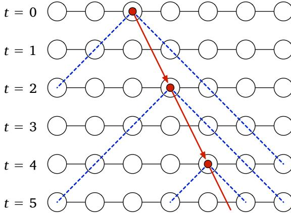
Figure 6.5: Algorithm APSP: the token walks along the BFS tree at speed 0.5 (thick arrows), while each  $\text{Wave}_v$  moves along the original graph at speed 1 (dashed lines). The waves are strictly nested: if  $\text{Wave}_v$  was triggered after  $\text{Wave}_u$ , it will never catch up with  $\text{Wave}_u$ .
