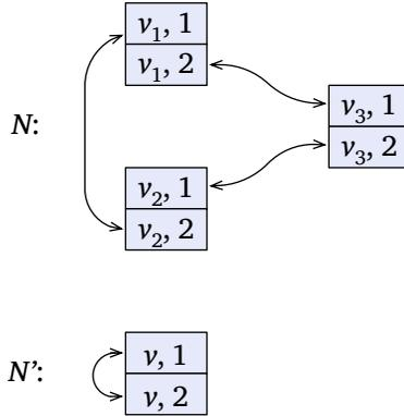
Figure 8.2: There is a covering map  $\phi$  from  $N$  to  $N'$  that maps  $v_i \mapsto v$  for each  $i \in \{1, 2, 3\}$ . Here  $N$  is a simple port-numbered network but  $N'$  is not.
