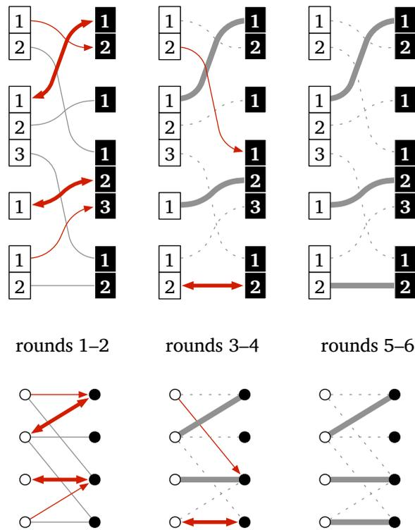
Figure 2.5: Algorithm BMM; the illustration shows the algorithm both from the perspective of the port-numbered network  $N$  and from the perspective of the underlying graph  $G$ . Arrows pointing right are proposals, and arrows pointing left are acceptances. Wide grey edges have been added to matching  $M$ .
