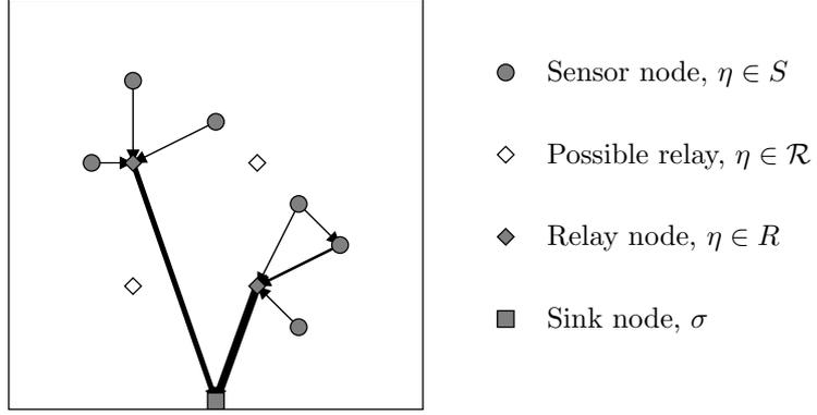
Figure 5: An instance of the relay placement problem. In this problem instance the set of possible relays was finite; there were 4 possible relays. Grey relays (2 in this example) illustrate one possible solution to the relay placement problem. Arrows illustrate corresponding data flows in the underlying balanced data gathering problem.
